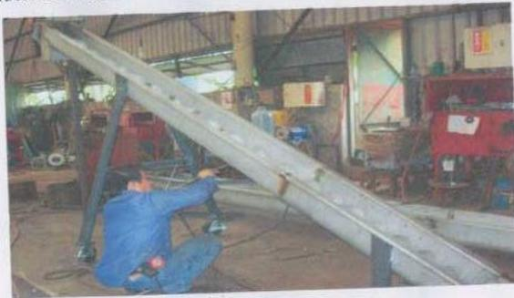
U型螺運機空機測試運轉
